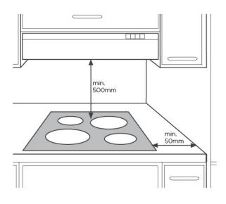
NOTE: The clearance must meet or exceed the minimum recommended for both the rangehood and cooktop. Refer to the rangehood installation manual.
